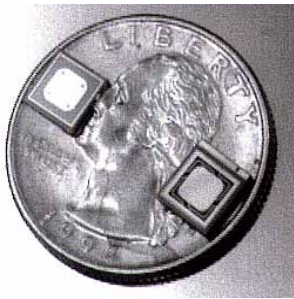
Figure 2. Photograph of the MEMS accelerometer die (without cap wafer).
