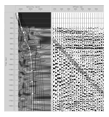
Figure 3. Velocity analysis for a shot gather treated as a pseudo-CDP gather. The white line is the picked stacking velocity, the black line indicates the velocities from the previous surface seismic line.
