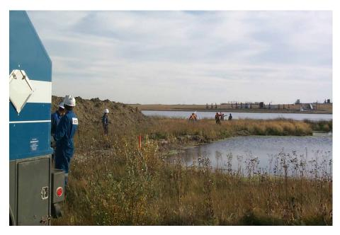
Figure 1. Deployment of the wireline across the "lake". The 5-level, 3-C VSP tool was attached at the far side of the lake and winched back to provide different receiver positions for the onshore vibrator.
