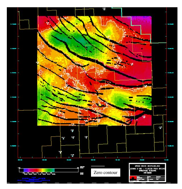
Figure 1. Difference map between Stacking velocity based model and Instananeous Velocity Model
