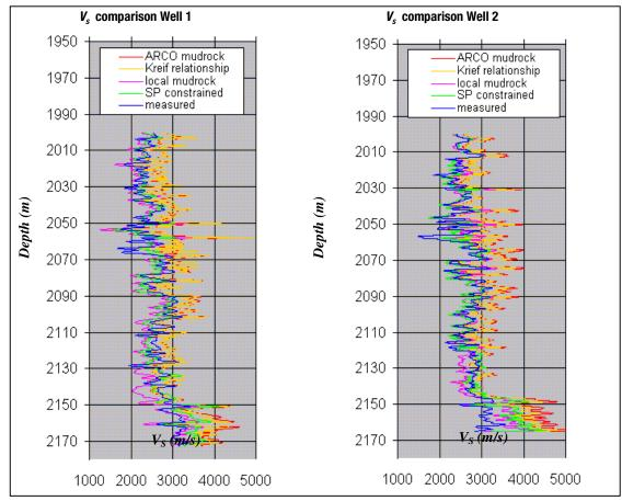
Figure 1: Comparison of shear-wave velocity estimation for wells 1 and 2
