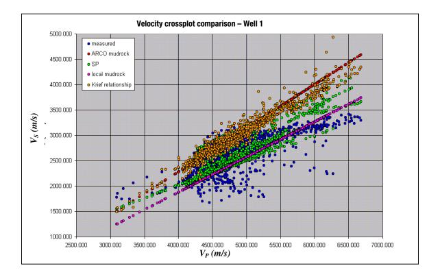
Figure 2: V<sub>p</sub> vs. V<sub>s</sub> crossplot showing measured and estimated values for well 1
