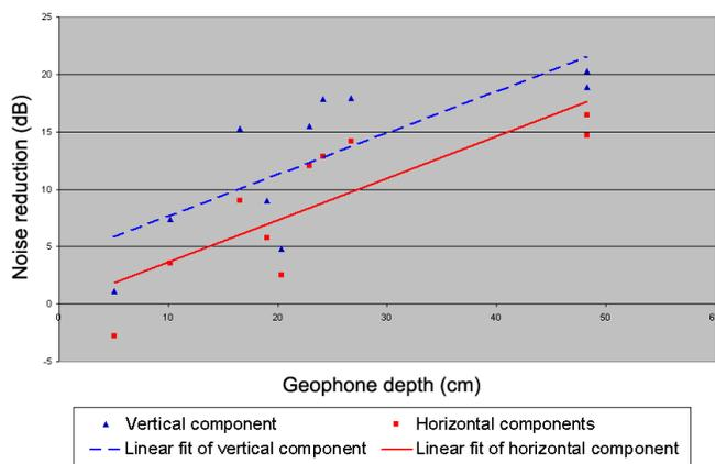
Figure 9. Noise reduction for buried geophones relative to a horizontal-component geophone planted on the surface.
