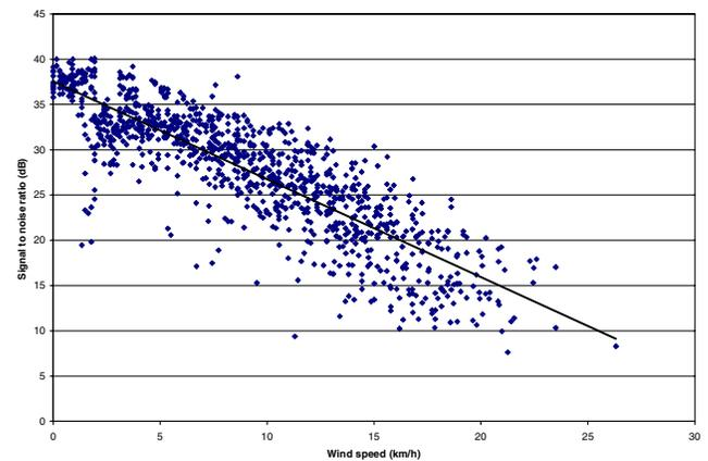
FIG. 5. Signal-to-noise ratio versus wind speed measurements obtained from a geophone buried 16.5 cm below the surface. The signal to noise ratio decreases linearly with wind speed.
