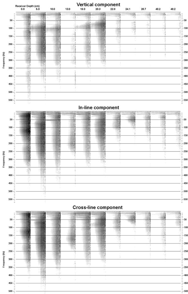
FIG. 7. A series of spectrograms for geophones at different depths. Each spectrogram is composed of power traces sorted by wind speed from 0 km/h to 22.5 km/h (left to right).
