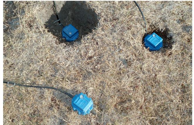
FIG. 8. Geophones were placed on the surface, and buried in holes of different depths. The figure shows holes of 18cm (top), 5 cm (right), and 0 cm (bottom).
