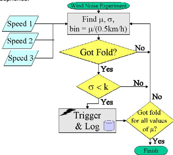
FIG. 3. Flowchart for the software that monitors the anemometers and triggers the recording geophone records. The procedure is based on the mean wind speed for all anemometers ( $\mu$ ) and the standard deviation between anemometer measurements ( $\sigma$ ).
