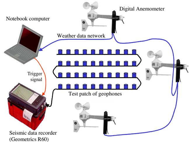
FIG. 1. Apparatus used to perform the wind-noise experiment.
