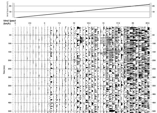
FIG. 4. Traces acquired by a single geophone element over a range of wind speeds. The equally gained traces shown an increase in background noise as the wind speed increases.
