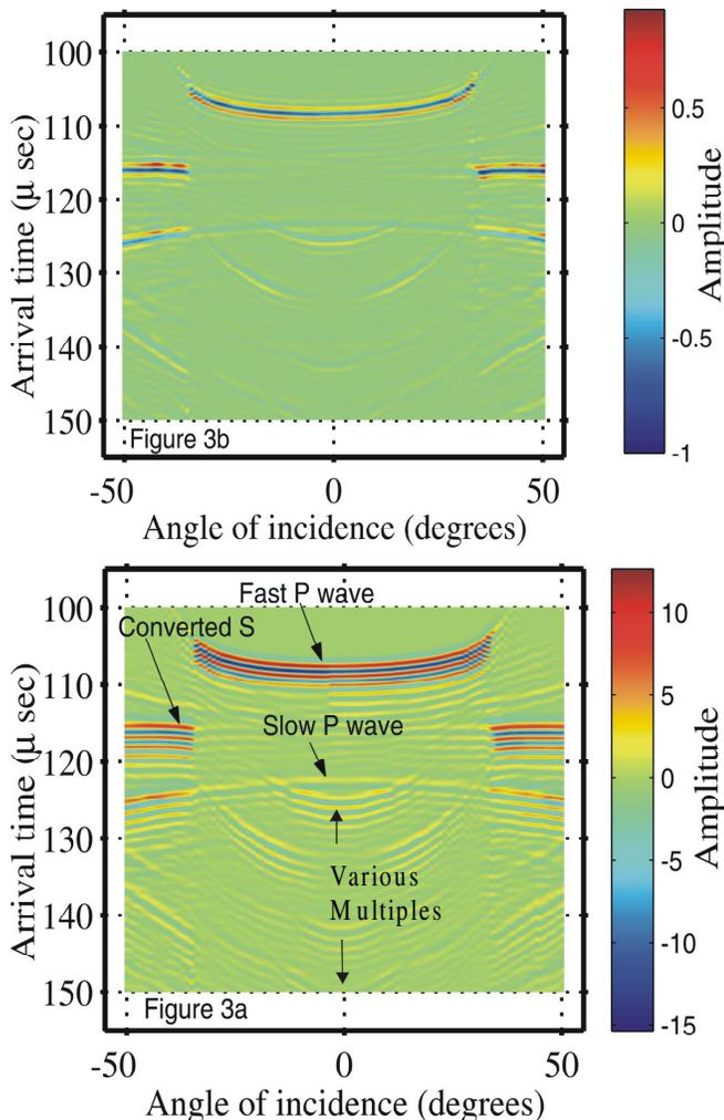
**Figure 3b:** The transmitted wavefield with a Minimum Entropy deconvolution applied. The waveform is greatly contracted and events have better continuity.
