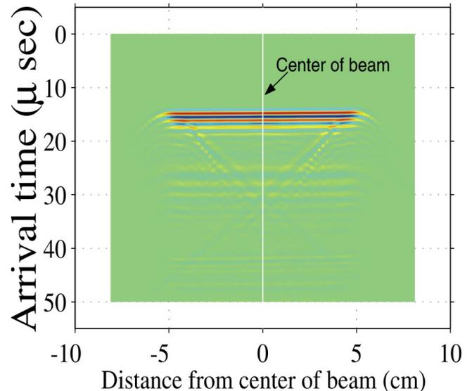
**Figure 2a:** The ultrasonic acoustic wave field as measured at normal incidence 2-cm away from the source. The source is kept fixed while the near-point receiver scans horizontally. The beam is flat (arrival time) in a range of about 10-cm.
