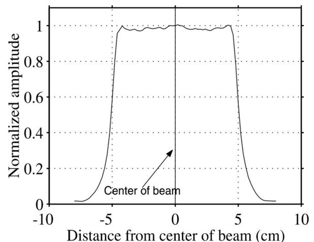
**Figure 2b:** The amplitude envelope of the ultrasonic acoustic wave field as measured at normal incidence 2-cm away from the source. The amplitudes are nearly constant in a range of about 9-cm.
