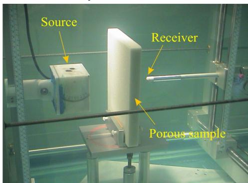
**Figure 1:** Experimental set-up for transmission through porous plate. A large area transducer (10-cm x 7.5-cm) as a source and a near-point receiver are used here. The porous synthetic sample is used. The angle of incidence is varied by a rotation of the porous plate. All the set-up is immersed in water.
