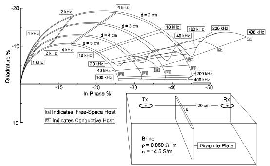
Figure 1. Complex space anomaly index diagram of the response of a thin vertical plate conductor to a two coil moving source EM system. Responses with a free-space host then with a conductive host are presented.
