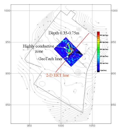
Figure 3. Depth slice from 0.35 to 0.75 m after inversion of 3-D ERT data.
