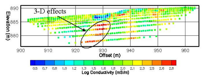
Figure 2. Conductivity section after inversion of 2-D ERT line.
