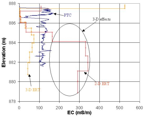
Figure 5. Vertical EC profile results from 2-D ERT and 3-D ERT inversions and PTC measurement.
