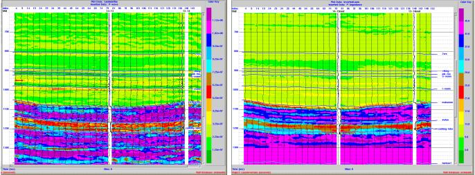
Figure 1: On the left is  $\lambda \rho$  calculated using Goodway's method. On the right is  $\lambda$  calculated using the new direct method. As expected, the  $\lambda \rho$  plot is noisier than the new inversion for  $\lambda$ . Inserted in the sections are  $\lambda \rho$  and  $\lambda$  logs at two well locations for comparison.
