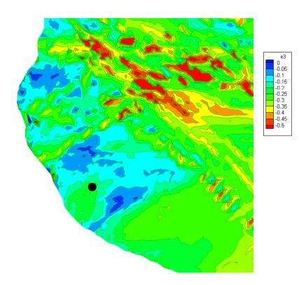
Fig 4 Strain values from three-dimensional reconstruction over the overthrust block at Circle Ridge field, Wyoming.
