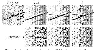
Figure 3: Inline slice through a noisy artificial volume showing the effects of eigenimage filtering with different values of *k*. Filtering becomes harsher as *k* decreases. Although k = 1 has removed most of the noise, the difference plot (the removed energy) shows it has also removed the weaker event. The result for k = 2 is more acceptable.
