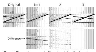
Figure 4: The exactness property. Shown is an inline slice through an artificial volume with four events but only three distinct dips.Eigenimage filtering with *k*=3 does nothing to the original data since the number of eigenimages equals the number of distinct dips.
