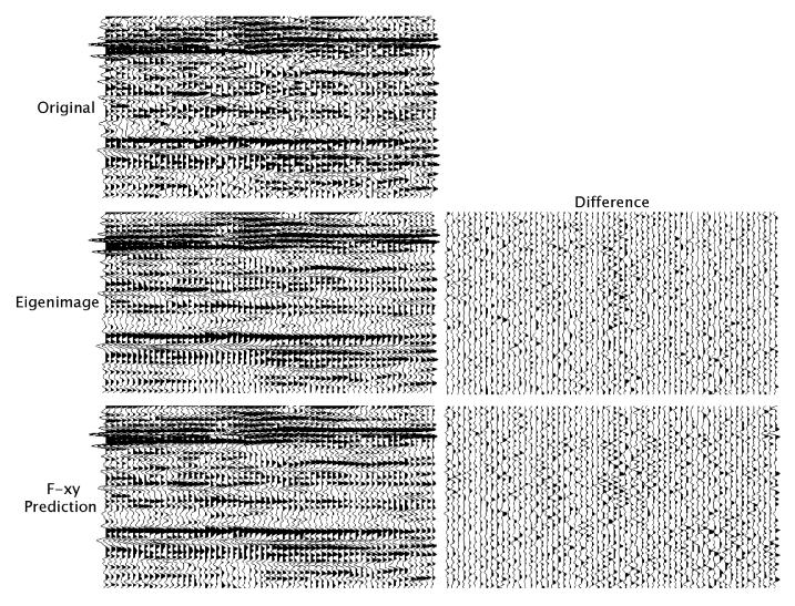
Figure 5: Real data example along an in-line slice comparing eigenimage filtering with k = 2, and f-xy prediction filtering with a 5x5 operator. There is little to choose between them using these parameters. Neither has remove much coherent signal.
