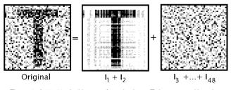
Figure 2: A 48x48 pixel image of a noisy letter T decomposed into the sum of its first 2 weighted eigenimages, containing most of the signal, and the sum of the remaining 46 eigenimages, containing most of the noise.
