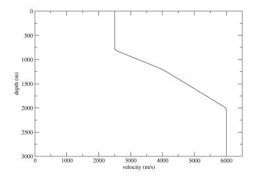
Fig. 3. Velocity in depth.
