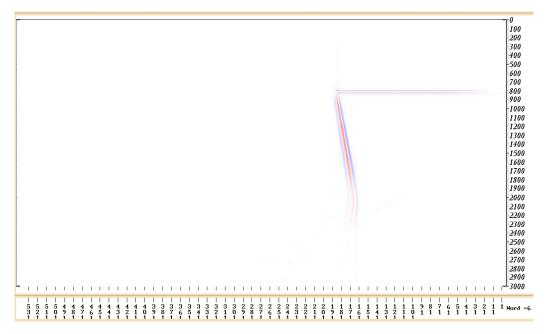
Fig. 5. Prestake migrated image in depth (converted from that in time).
