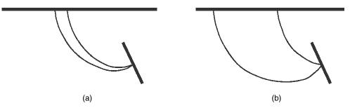
Fig. 1. Imaging dips beyond 90 degrees by seismic turning waves: (a) near offset case where both incident and reflected waves are turning waves; (b) far offset case where only one (but not both) of the incident and reflected waves is a turning wave.
