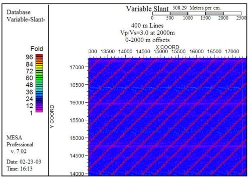
Variable Line Spacing, Slante Shot Line Design – Vp/Vs = 3.0 at 2000 m depth
