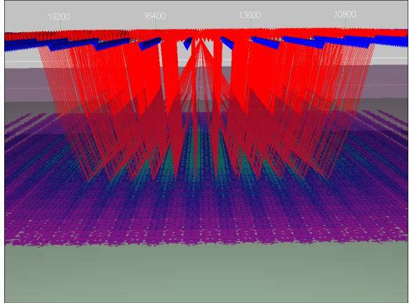
Converted Wave Rays in Layered Model
