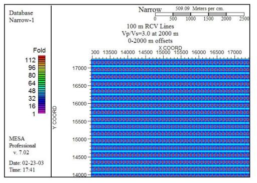
Narrow Azimuth Design – Vp/Vs = 3.0 at 2000 m depth
