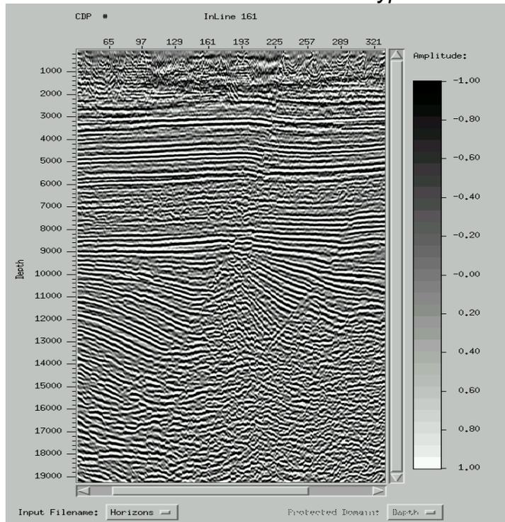
Fig. 5: Two-way migration of a South Texas land data set. The velocity model used for this migration was identical to the one used to obtain Fig. 4.
