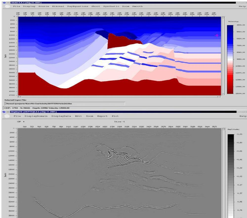
Fig. 1: Top is a velocity model of a Gulf of Mexico Salt Structure. Bottom is a one-way migration of synthetic data calculated from the model.
