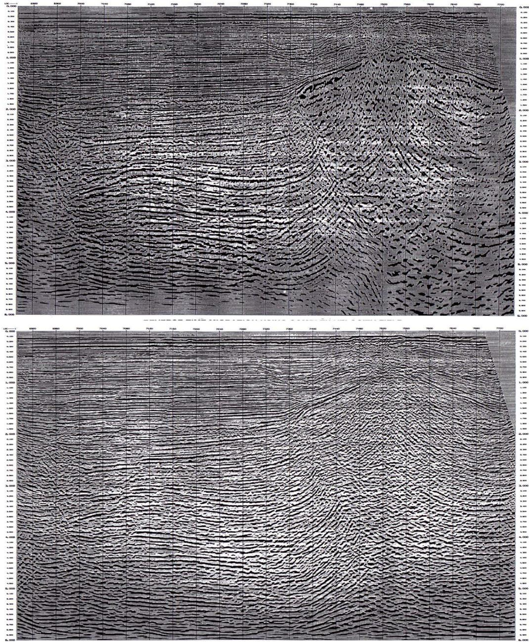
*Fig. 3: Two-way vs. one-way migration of a Gulf of Mexico salt structure. Top is a full two-way migration. Bottom is a one-way steep dip migration of the same structure. Note: top is the same image as in Figure 2.*
