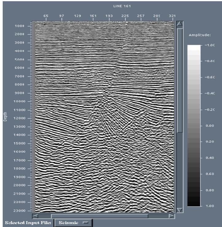
Fig. 4: One-way maximum amplitude Kirchhoff migration of a South Texas land data set. This line demonstrates the resolution of a typical fault shadow problem.
