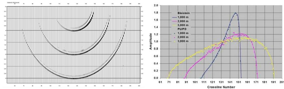
*Fig. 2: Left: 3-D phase-shift migrated impulse responses along the center inline. The shot is at crossline 121 and receiver at crossline 141. Right: Amplitudes of the 3-D migrated impulse responses.*
