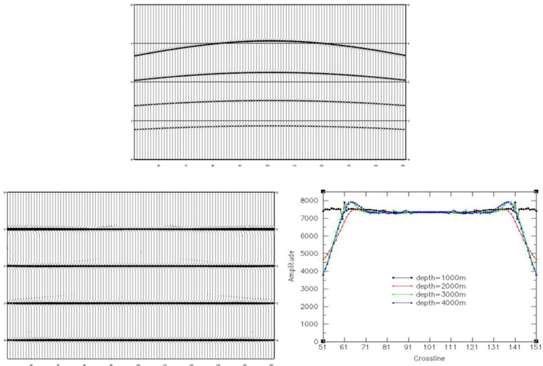
Fig. 5: Top: 2-D shot record from four flat reflectors in a medium with velocity  $v(z) = 2000 + 0.3z$ . Bottom left: migrated shot record. Bottom right: Peak amplitudes along the migrated reflector.
