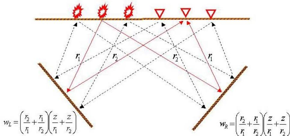
*Fig. 3: Ray density for common-offset migration onto dipping reflectors.*
