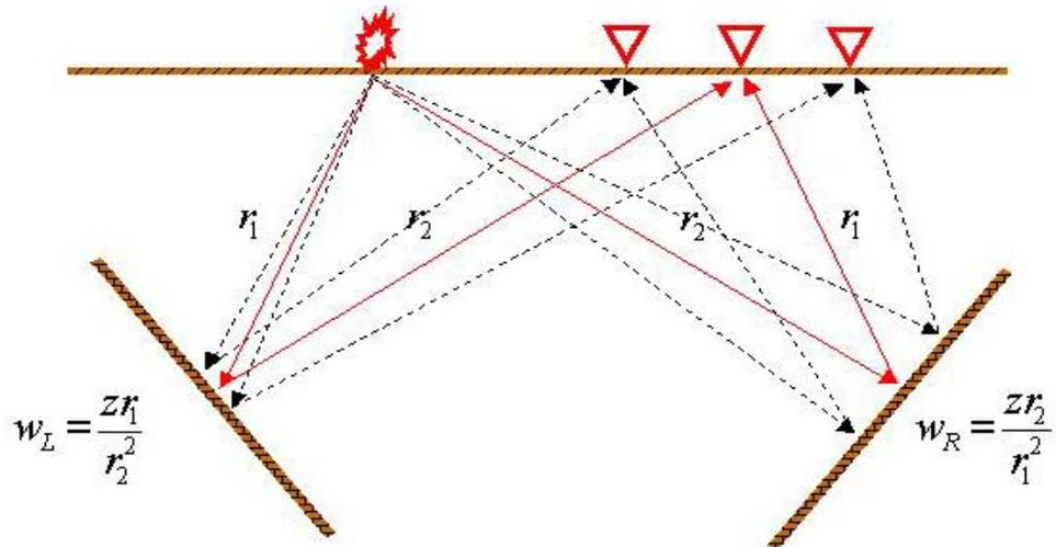
Fig. 4: Ray density for common-shot migration onto dipping reflectors.
