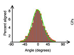
Fig. 1. Orientation distribution of clay platelets reproduced from the Hornby et al. (1994) and approximation by the normal distribution function.
