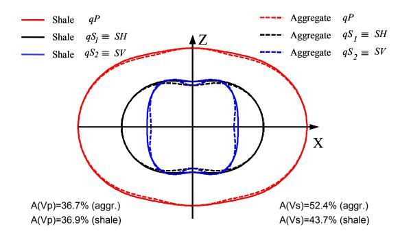
Fig. 3. Phase velocities of Chattanooga Shale from Johnston & Christensen (1995) and polycrystalline aggregate calculated from the geometric mean averaged elastic constants (Fig. 2).
