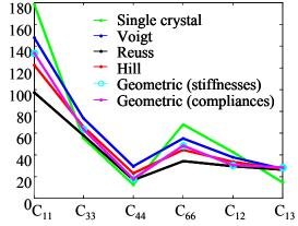
Fig. 2. Elastic constants of polycrystalline aggregate calculated with Voigt, Reuss, Hill and Geometric mean approximations. Single crystal elastic constants are shown for comparison.
