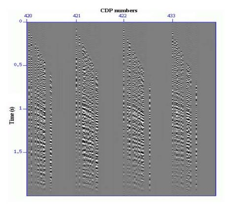
Fig. 1. CDP gathers for in-line #10, each gather has 60 offsets with a spacing of 25 meters.
