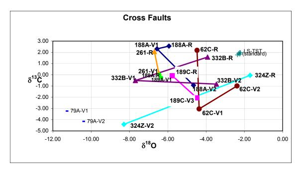
Fig. 3. Isotopic trends for samples collected from cross-fault zones. Veins within the cross faults tend to have an isotopic signature that is higher in  $\delta^{18}$ O and lower in  $\delta^{13}$ C than the host rock, indicating that the veins formed from a mixture of host-rock-derived fluids and formation waters. Samples 79A-V1 and 79A-V2 are included to illustrate a strongly meteoric signature.
