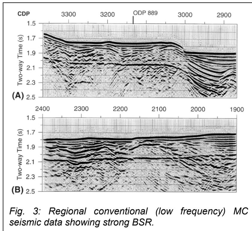
*Fig. 3: Regional conventional (low frequency) MC seismic data showing strong BSR.*
