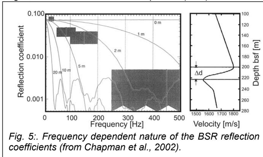
Fig. 5: Frequency dependent nature of the BSR reflection coefficients (from Chapman et al., 2002).
