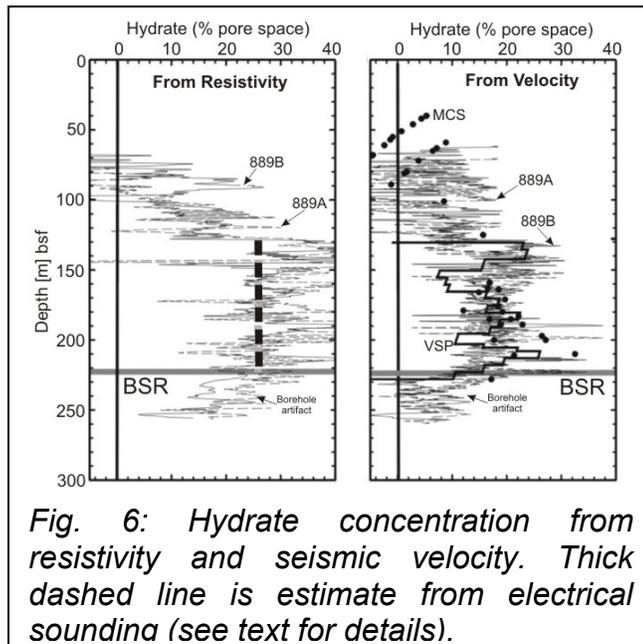
*Fig. 6: Hydrate concentration from resistivity and seismic velocity. Thick dashed line is estimate from electrical sounding (see text for details).*
