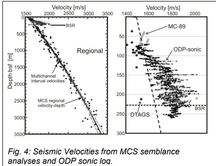
Fig. 4: Seismic Velocities from MCS semblance analyses and ODP sonic log.
