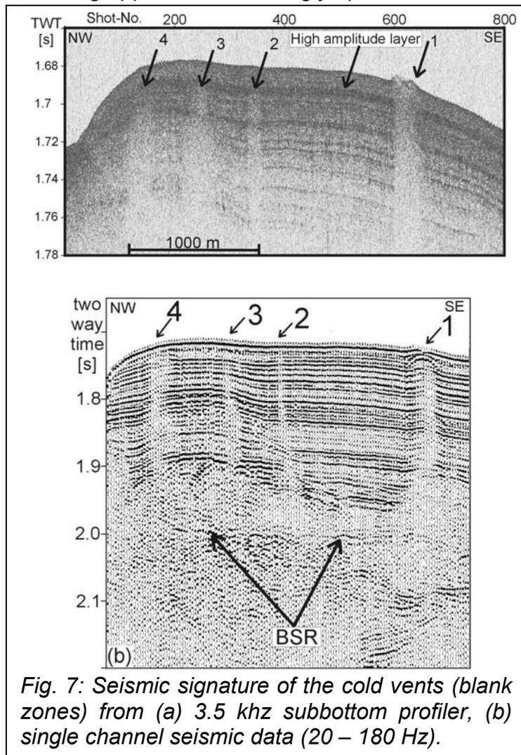
Fig. 7: Seismic signature of the cold vents (blank zones) from (a) 3.5 khz subbottom profiler, (b) single channel seismic data (20 – 180 Hz).
