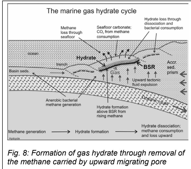
*Fig. 8: Formation of gas hydrate through removal of the methane carried by upward migrating pore*
