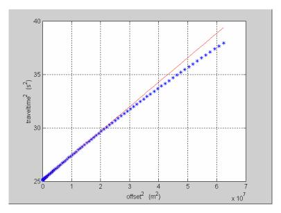
Fig. 8. The  $t^2 - x^2$  curve shows nonhyperbolic moveout in multi-layered VTI media. The straight line is used to obtain the short-spread converted NMO velocity,  $V_c = 2134 \text{ m/s}$ .
