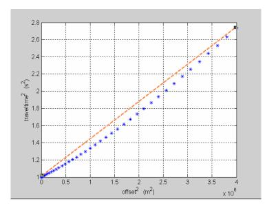
Fig. 3. The  $t^2 - x^2$  curve shows nonhyperbolic moveout.
