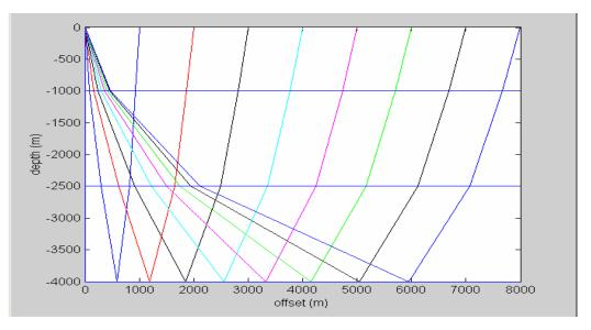
*Fig. 7. The P-S wave raypaths generated from the three-layered VTI model using Thomsen's exact equations.*
