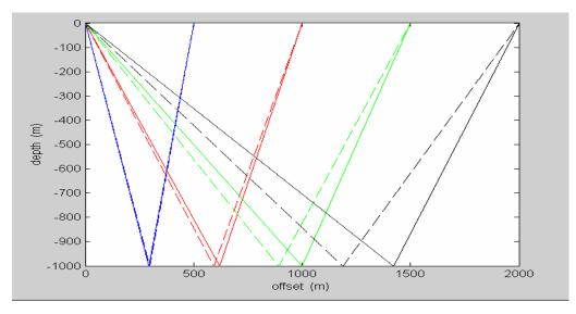
Fig. 4. This figure displays the raypaths and the corresponding conversion point location generated from two methods. The solid lines represent the conversion point location obtained from Thomsen's exact equations, where the dashed line represents the position obtained from  $\gamma_{eff}$  method.
