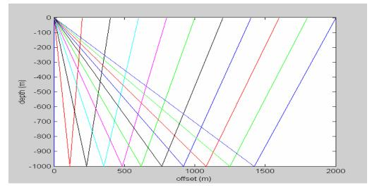
Fig. 2. The raypaths of the P-S converted wave, for a series of offsets, generated from the one layer VTI model shown in Figure 1, using the exact equations.
