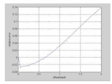
Fig. 10. The relative error of the conversion point at the base of 3-layer model obtained from the effective velocity ratio method.
