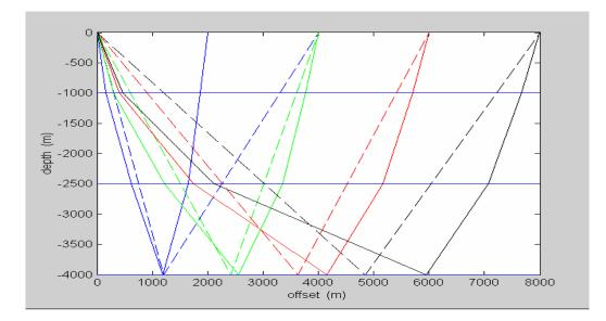
Fig. 9. The P-S conversion-point position obtained from two methods being applied on the three-layer VTI model. The solid lines show the ray path for certain offsets generated from Thomsen's exact equations and the dashed lines show the conversion-point position by effective velocity with  $\gamma_{eff} = 1.384$ .
