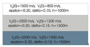
Fig. 6. A three-layer VTI model in with properties defined as shown.
