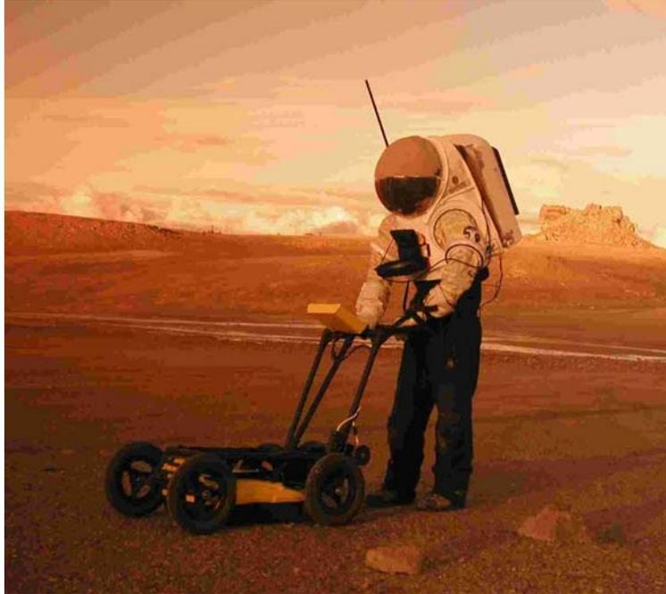
*Fig 9. GPR system NOGGIN 250 MHz System being used at the Von Braun Valley site. R. Birch is shown testing a prototype space suit.*
