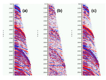
Fig. 4: (a) Input CMP, (b) input CMP with second order deconvolution operator applied in tau-p domain, and (c) difference between (a) and (b).
