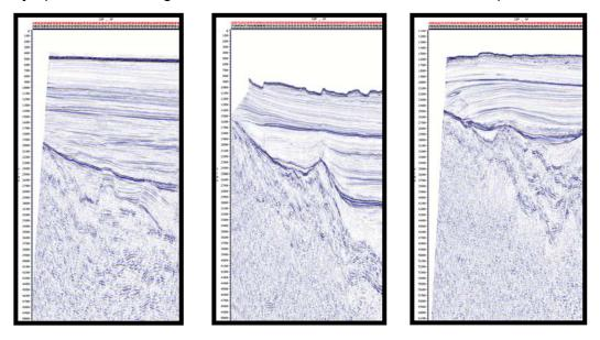
*Fig. 7: Final migrated stacks of test lines after full demultiple application. See fig. 1 for comparison.*
