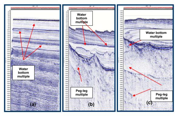
*Fig. 1: Test line stacks from one survey demonstrating varied and severe multiple problems.*
