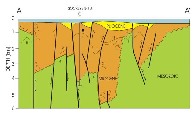
Fig. 4. Simplified structural cross-section for offshore region of Hecate Strait; from Hannigan et al. (1998), modified after Dietrich (1995). Location of line of cross-section shown on Fig. 1.
