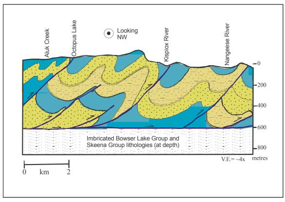
Fig. 3. Schematic structural cross-section across Kispiox River valley, north-central 93P/09.
