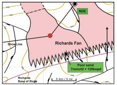
multiple stacked and offset channel/ levee/ fan deposits with a combination structural drape and stratigraphic pinchout forming the trap. An offset well on the southern fringe penetrated a portion of the fill and tested 7 MMCF/d & 120 BOPD from an Upper Richards channel sand. AVO indicates probable gascharged sands within this upper Richards complex. Worldwide analogies
