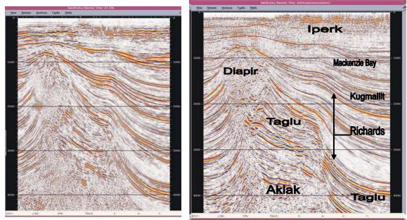
Figs. 1 & 2: Shale Diapir on old 2D (left) and new 3D (right) seismic data
