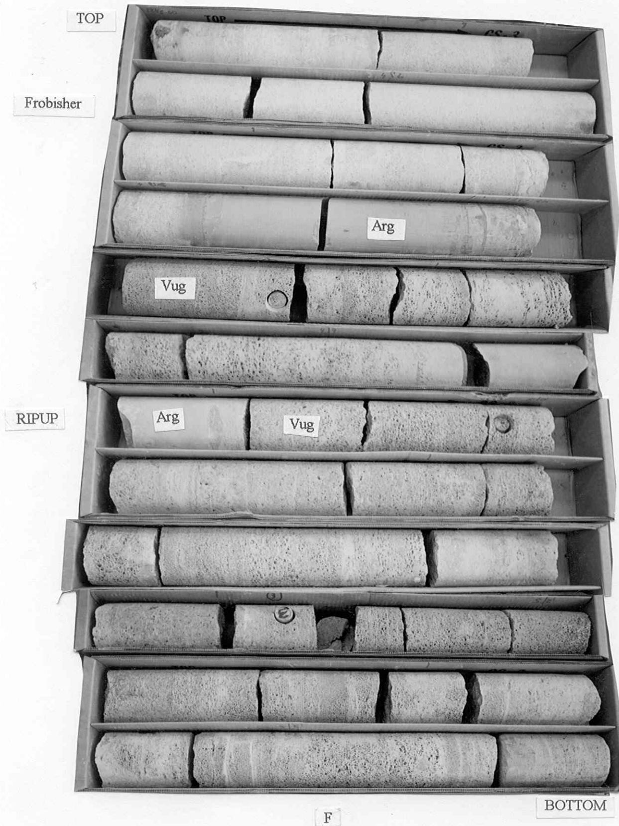
Cycles within the Frobisher Lowstand Systems Tract. Individual cycles consist of highly argillaceous mudstones (erosional bases –Arg) which grade into vuggy porosity limestones (Vug). Note ripup clast (with vuggy porosity development) incorporated into the argillaceous base of the cycle. (Details of this feature in the following core photo). (2D14-34-3-1W2M, 1245-1253m).
