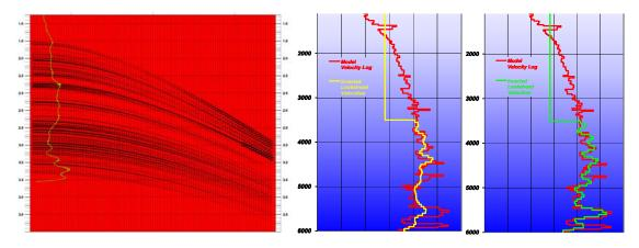
Figure 2. East coast synthetic walkaway with moveout inversion results showing smoothly varying velocity trends. Sufficient offset aperture is important for velocity sensitivity.
