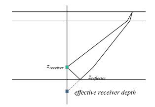
Figure 1. Schematic of the procedure to transform an offset VSP reflection ray path into a direct ray-path so that effective VTI theory can be used. Layered model parameters are mirrored about the reflector depth and the actual receiver depth is replaced by a new effective receiver depth.
