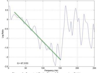
Figure 3. Spectral Ratio Plot of Downgoing P-Wave
