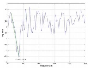
Figure 6. Spectral Ratio Plot of Downgoing S-Wave
