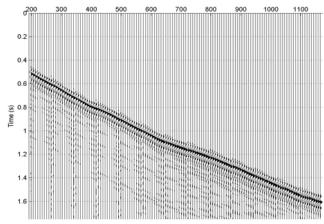
Figure 4. Downgoing S-Wave (depth(m) vs. time(s))
