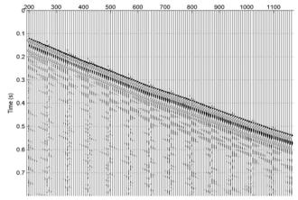
Figure 1. Downgoing P-Wave (depth(m) vs. time(s))
