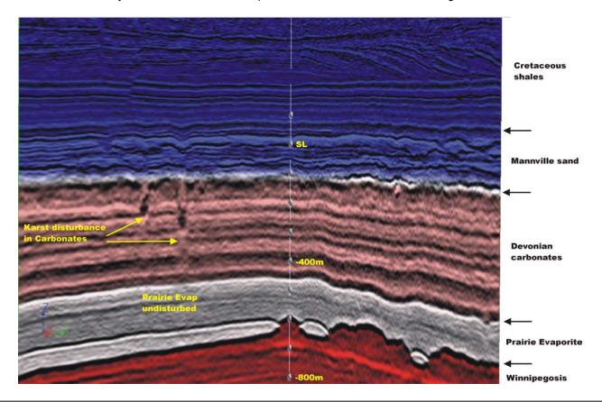
Figure 3: Another fence from the Allan data volume; this section has a 2X vertical exaggeration. Two Karst-type disturbances are marked; these features are about 130 – 150 m wide.
