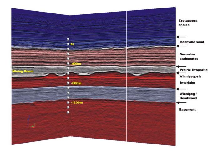
Figure 2: PSPI depth-migrated seismic section showing normal central Saskatchewan stratigraphy (from the Allan area); section has a 2X vertical exaggeration. This is a different view of the data shown in Figure 1. Fence sections are painted with velocity from the model derived during the migration: blue is slow (shales & sand), red is fast (carbonates & basement), and grey is intermediate-speed (salt & sand).
