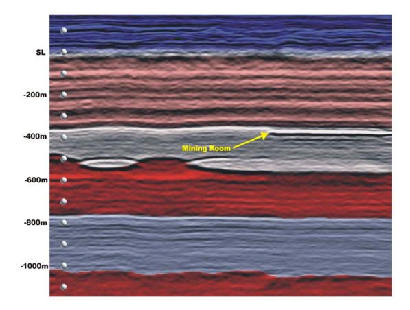
Figure 1: PSPI depth-migrated seismic section in metres below Sea Level (SL); this section has a 2X vertical exaggeration. The arrow marks a "cultural" reflector, Allan mine Panel N2E.
