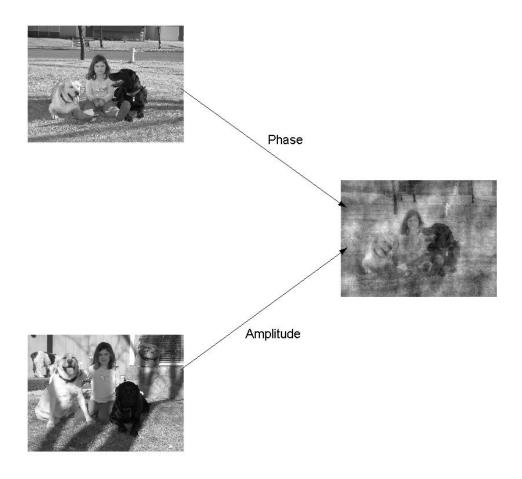
Figure 3: The phase of one image is combined with the amplitude of another to create a new image. The resultant image is most similar to the image with the same phase.
