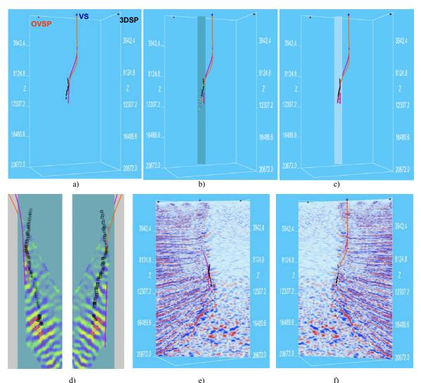
Figure 4. a) Source locations of Offset VSP, Salt Proximit, and Velocity Survey and multiple well paths as well as salt exit points (black dots). b) Salt exit points superimposed on updip sand images. c) Depth migration image of salt-sediment boundary vs. salt exit points. d) salt exit points, sediment image and well paths are displayed from the front and back. e) Front and f) back display of surface seismic section, salt exit points, and well paths.
