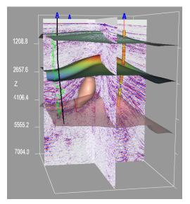
Figure 1. 3D visualization of seismic volumes, complex geological structures, layer-velocity model, log curves in multiple wells.
