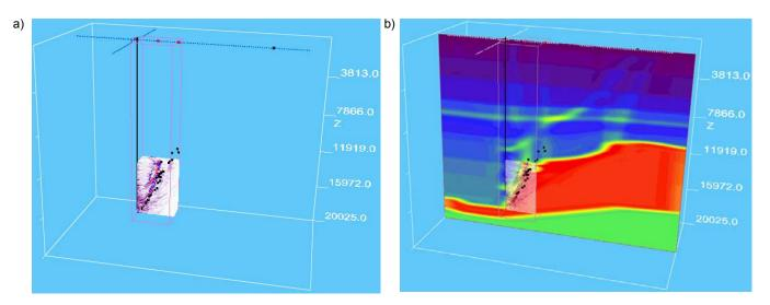
Figure 3. a) Survey geometry with vertical well and seismic sources of the offset VSP (red dots), salt proximity(Black dot), and walkaway VSP (blue dots). 3D salt exit points are superimposed on 3D images of depth migration cube. b) Visual Integration of 3D depth migration volume, salt exit points, and velocity distribution from traveltime tomography.
