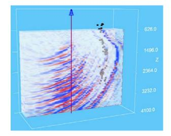
Figure 2. 3D VSP migration volume showing images of the overhanged salt-sediment boundary and the updip sediments. Black dots are salt exit points derived using a salt proximity method. The vertical line indicates location of wellbore.
