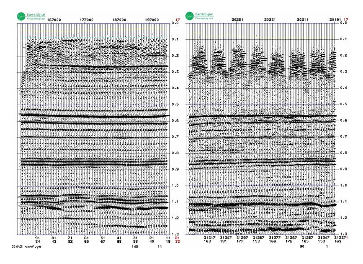
Figure 4: Stack section. Weight drop (left) and dynamite (right)
