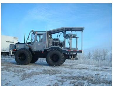
Figure 1: Surface weight drop unit.
