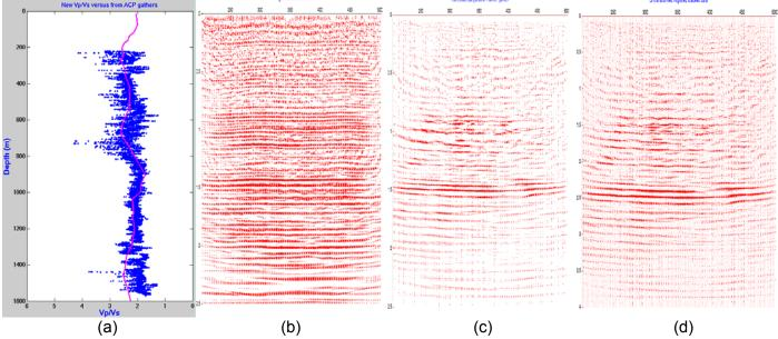
Figure 4. From left to right are: (a) the comparison of the scanned  $\gamma_0$ -log (pink curve) and the  $\gamma_0$ -log from the Well-09-08 (blue curve); (b) PP stacked data; (c) transformed PS data using the scanned  $\gamma_0$ -log: the scanned  $\gamma_0$ -log was smoothed before using it to transform PS to PP time. (d) The untransformed PS stacked data. Note the difference in the time scale between (c) and (d).
