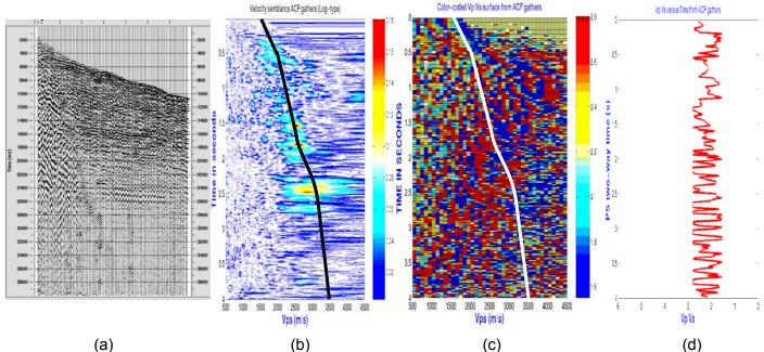
Figure 3. From left to right are (a) seismic ACP gather, (b) 2D velocity semblance, (c)  $\gamma_0$ -panel on which is superimposed the picked velocity function, (d)  $\gamma_0$ -time log that is automatically plotted.
