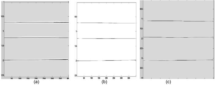
Figure 2. PS to PP time mapping. From left to right are (a) PP stacked data, (b) transformed PS to PP time stacked data, (c) untransformed PS stacked data. Note the difference in time scale between (b) and (c).
