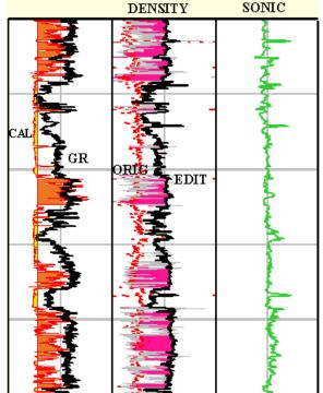
Figure 4. Example of curve reconstruction for density in washed out shales. In track 2, original Rhob is gray, edited Rhob is black.
