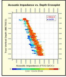
Figure 3. Acoustic impedance trends for Niterk L-19 show sands have lower impedance than shales
