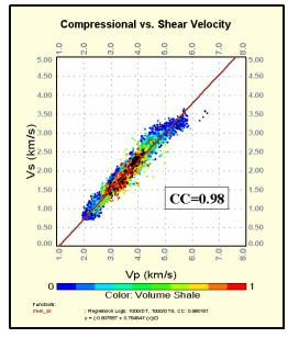
Figure 5. VpVs relationship for BMB based on 5 wells with measured shear data.
