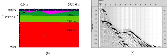
Figure 2. (a) Velocity model used for case I. (b) The synthetic shot gather.
