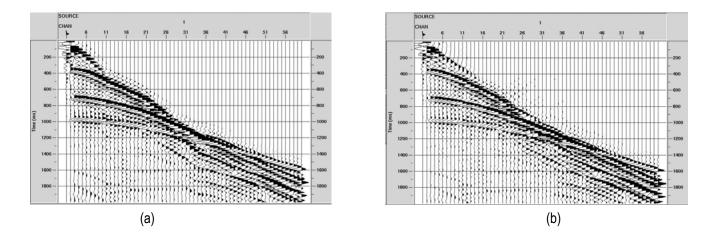
Figure 5. (a) After applying vertical static shifts to move the data to a flat datum. (b) After wave equaiton datuming. Note that wave equation datuming result is superior to the vertical staic shifts where raypaths are not near the vertical (Case II).
