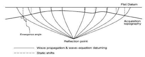
Figure 1. A comparison between wave equation datuming and vertical static shifts (taken from Bevc (1997)).
