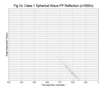
Fig.2b: AVO-Class 1 Spherical Wave PP Reflection Coefficient
