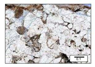
Figure 1: This section of a formation between 13880 and 13900 feet indicates that the rock type exhibited the lowest shale content but the pervasive quartz cement affects reservoir quality.
