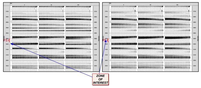
Figure 4: Synthetic gathers generated with a (a) 60 hz wavelet and (b) 35 hz wavelet and indicated values of water saturation. Evidently, gathers with 60 hz exhibit amplitude variation with offset.
