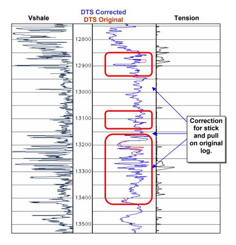
Figure 2: Stick-and-pull correction effected on the original log.
