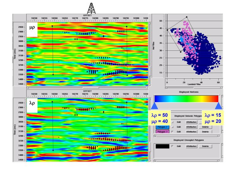
Figure 6: Lambda-Rho and Mu-Rho sections alongwith the associated cross-plot. A polygon on the crossplot loghts up the prospective zones on the two sections.
