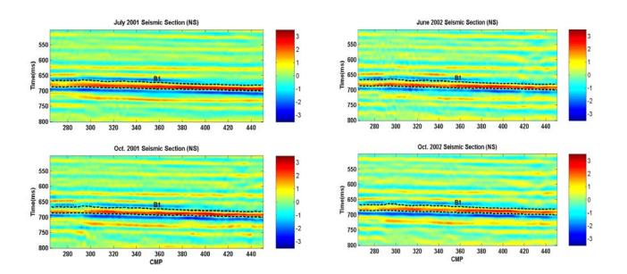
Figure 5 Four time-lapse seismic sections acquired at different times
