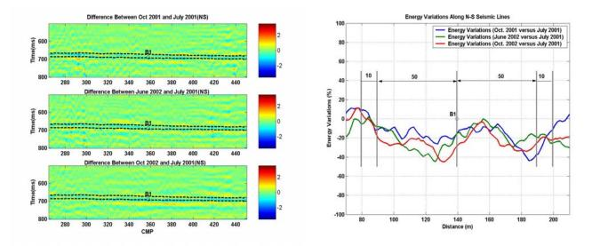
Fig.6 Amplitude difference and energy variations within the defined window along N-S seismic line direction. The data from July2001 was used as slave survey, the remaining surveys as monitoring surveys.
