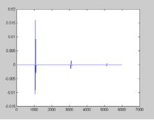
FIG. 5. The Q-filtered seismic trace with Q=70.
