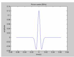
FIG. 1. Ricker wavelet with a dominant frequency of 50 Hz.
