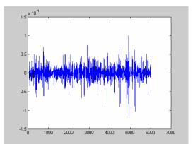
FIG.8. The seismic trace formed by convolving 50 Hz Ricker wavelet with random reflectivity.
