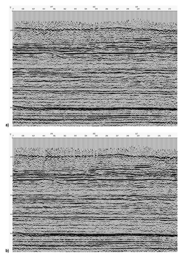
Figure 2. Vertical data stacked with PP velocity. (a) DSU3. (b) VectorSeis®.
