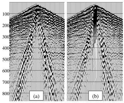
**Figure 1.** Prestack data comparison: (a) shot profile of DSU3 data. (b) VectorSeis<sup>®</sup> data of the same shot location. The full scale of MEMS (a) is about twice that of MEMS (b) and its recovery time from overdrive is much faster. As a result, overdrive is more apparent on (b).
