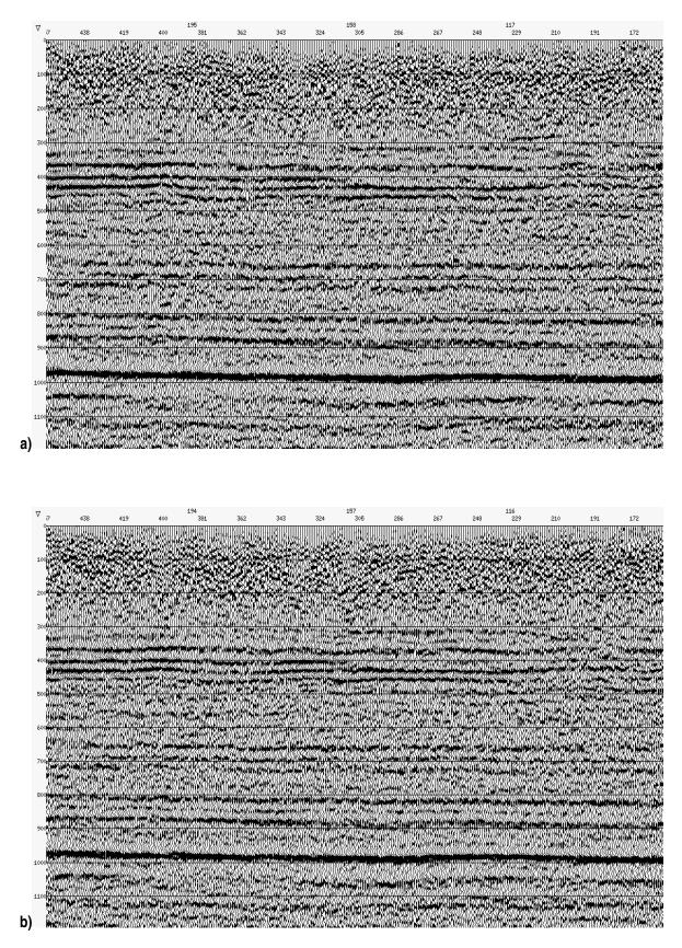
Figure 3. Radial data stacked with PS velocity. (a) DSU3. (b) VectorSeis®.
