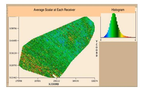
Figure 4. Map and histogram of the QC scalars, which are the average of the scalar traces at each receiver location. Poorly coupled receivers can be seen in the map and in the histogram as anomalously high values.
