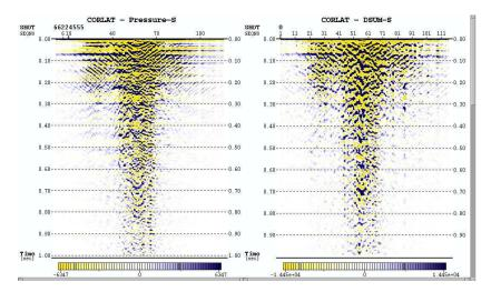
Figure 3. Autocorrelations of the hydrophone data (on the left) and the summed data (on the right).
