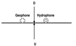
Figure 1. The upgoing and downgoing waves are recorded by the hydrophone and vertical geophone on the seafloor.
