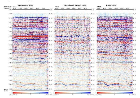
Figure 5. A comparison between the unsummed hydrophone (on the left) and vertical geophone data (in the middle) and the summed data (on the right).
