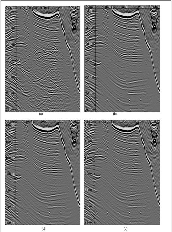
Figure 2: Zoom view of the area under salt bottom in Figure 1. (a), before multiple attenuation; (b), from data with no free surface multiple; (c) minimum energy wavelet extraction with four Taylor terms; and (d), 1D matching filtering.
