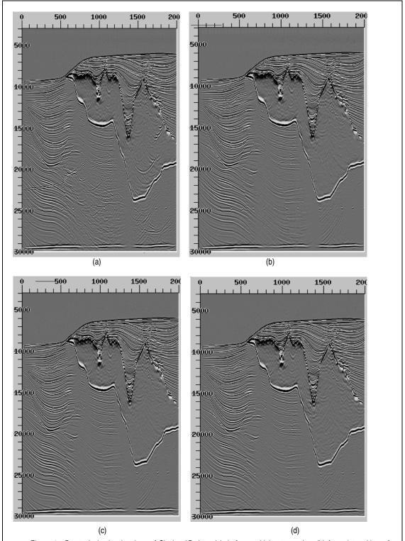
Figure 1: Prestack depth migrations of Sigsbee2B data. (a), before multiple attenuation; (b) from data with no free surface multiple; (c), minimum energy wavelet extraction with four Taylor terms; and (d), 1D matching filter.
