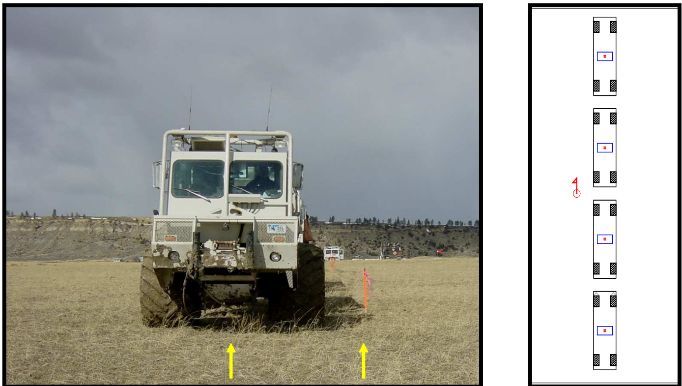
Figure 1. Inline vibrator positions. In the picture on the left, the vibrator operator must offset the unit in order to see the stake. The diagram on the right depicts an overhead view of an inline vibrator array showing the offset to the surveyed stake position.
