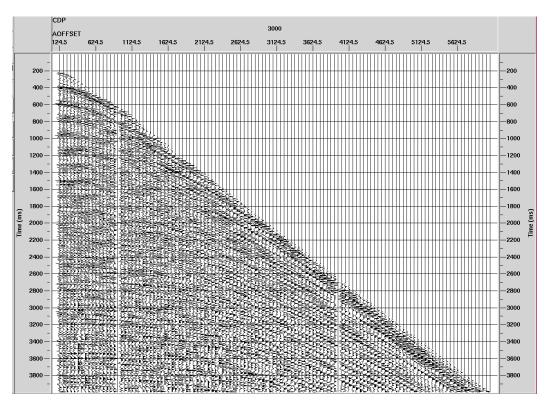
Figure 5 The input seismic CMP gather
