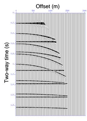
Figure 1 An NMO-corrected muted synthetic CMP data.
