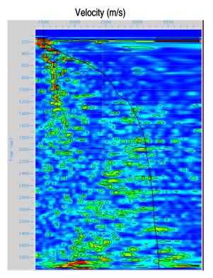
Figure 6 The semblance of the input CMP gather in Figure 5
