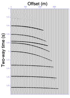
Figure 3 The reconstructed multiples in time-space domain.
