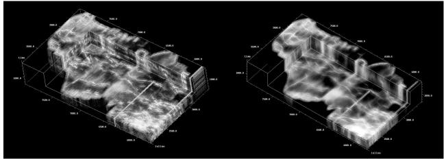
Figure 3: Left is a line enhanced relative probability volume. Right is a fault enhanced relative probability volume. Notice in particular the improved continuity and signal to noise ratio for faults on the vertical sections in the volume.
