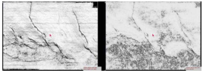
Figure 1: Modified EigenStructure on the left versus competitive "discontinuity" at right for time slices at 600 ms.
