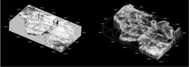
Figure 2: Left is a Coherency volume. Right is a line enhanced relative probability volume.
