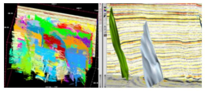
Figure 4: Left, all fault picks. Right, two selected fault surfaces.
