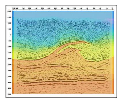
Figure 2: PreSDM Inline 320 with final velocity model overlay
