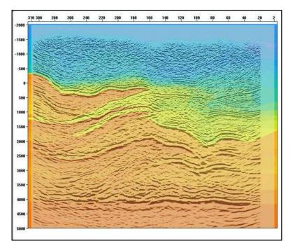
Figure 1: PreSDM Inline 120 with final velocity model overlay
