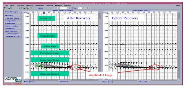
Figure 3 Synthetic seismograms generated from NORSAR3D seismic modeling
