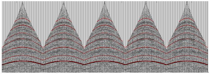
Fig. 1. High-density automatic traveltime picking
