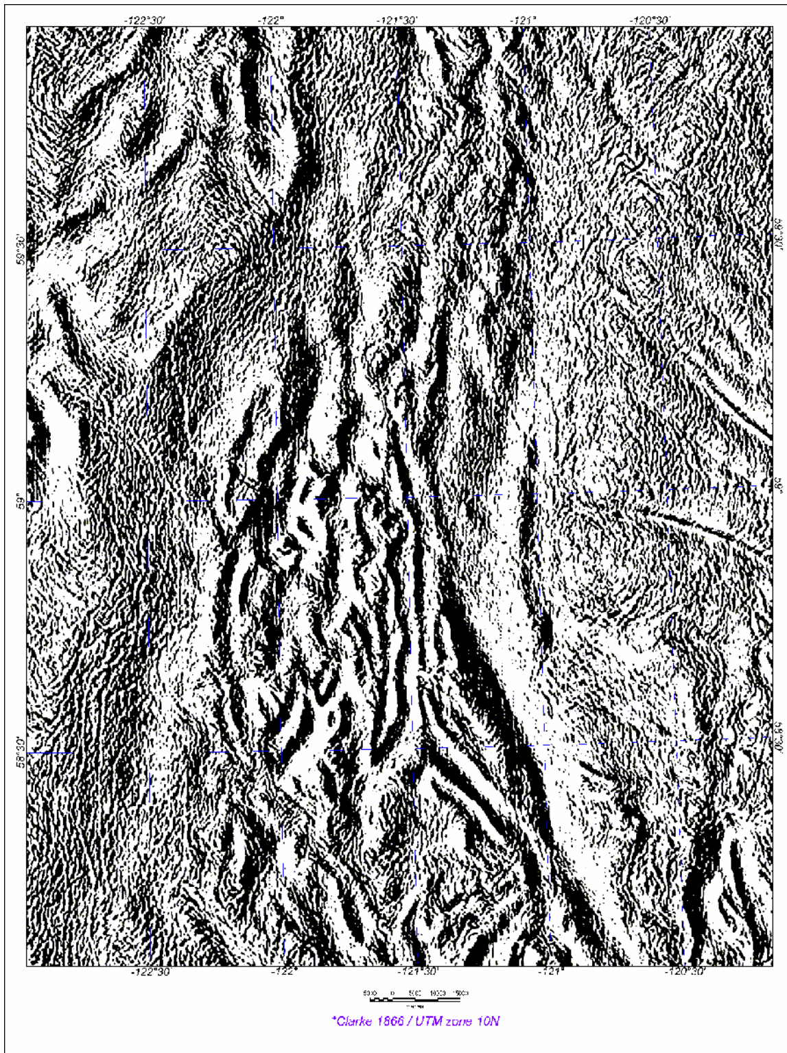
Figure 4. The result of 2-D wavelet transform showing the N-S lineaments of the area.
