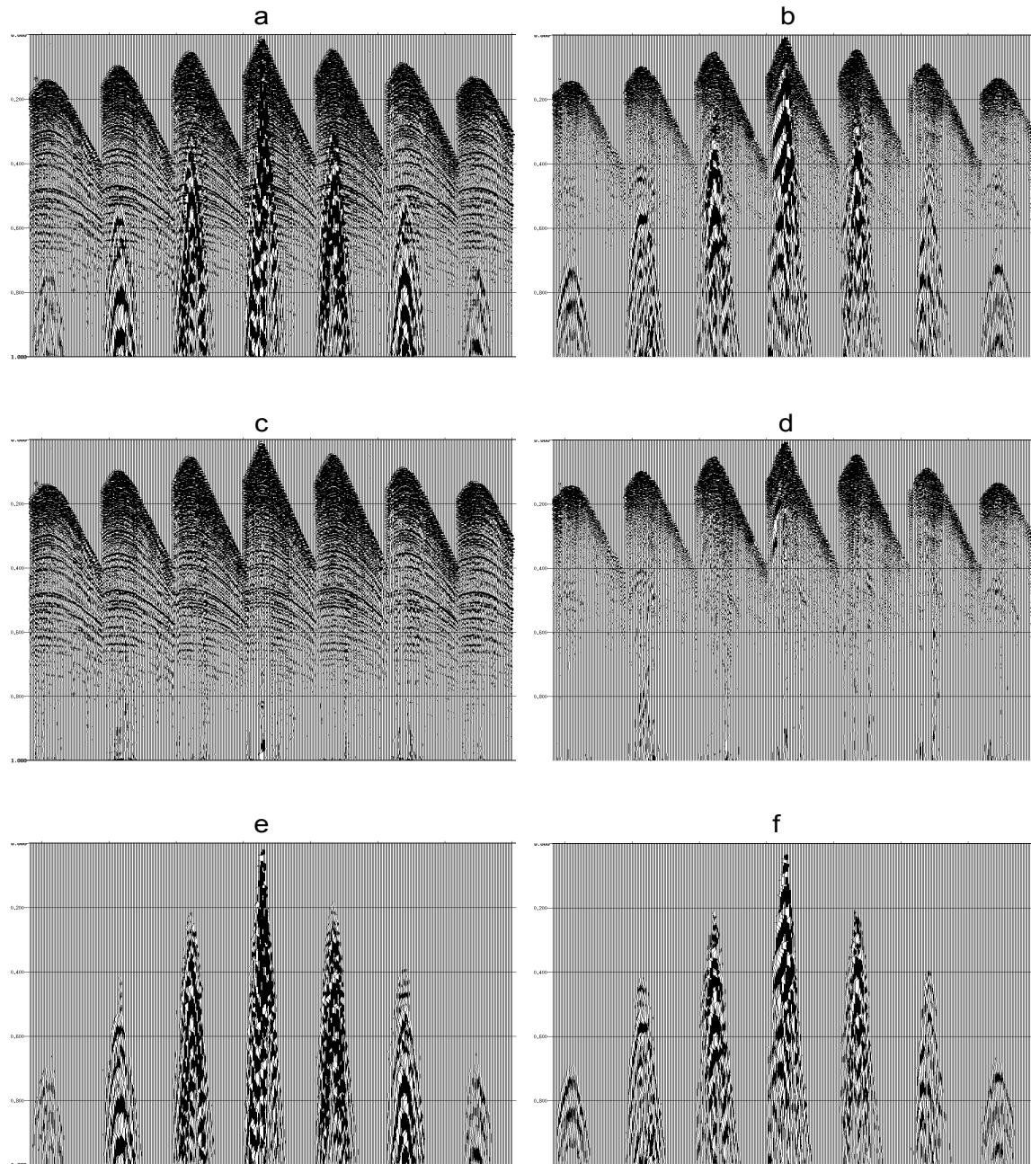
Figure 3. Results of polarization filter on a 3C 3D data: (a) raw shot records of vertical components, (b) raw shot records of radial components, (c) vertical components after polarization filter, (d) radial components after polarization filter, (e) difference of vertical components, (f) difference of radial components.
